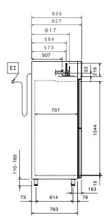
Electrical inlet (power) RI Refrigerant Inlet RO Refrigerant Outlet
